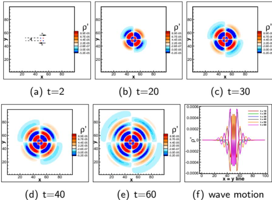
Figure: Density perturbation waves for the case of a lateral quadrupole
