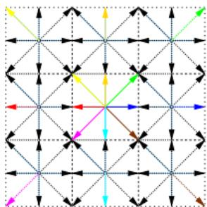
**Figure:** Schematic showing the streaming operation
