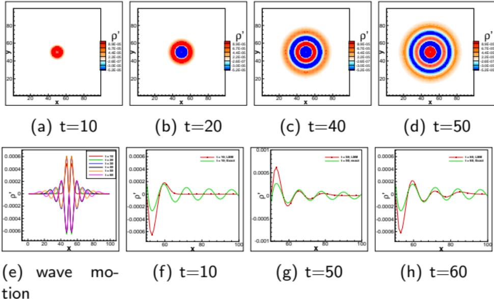
**Figure:** Propagation of density perturbation waves for the case of monopole
