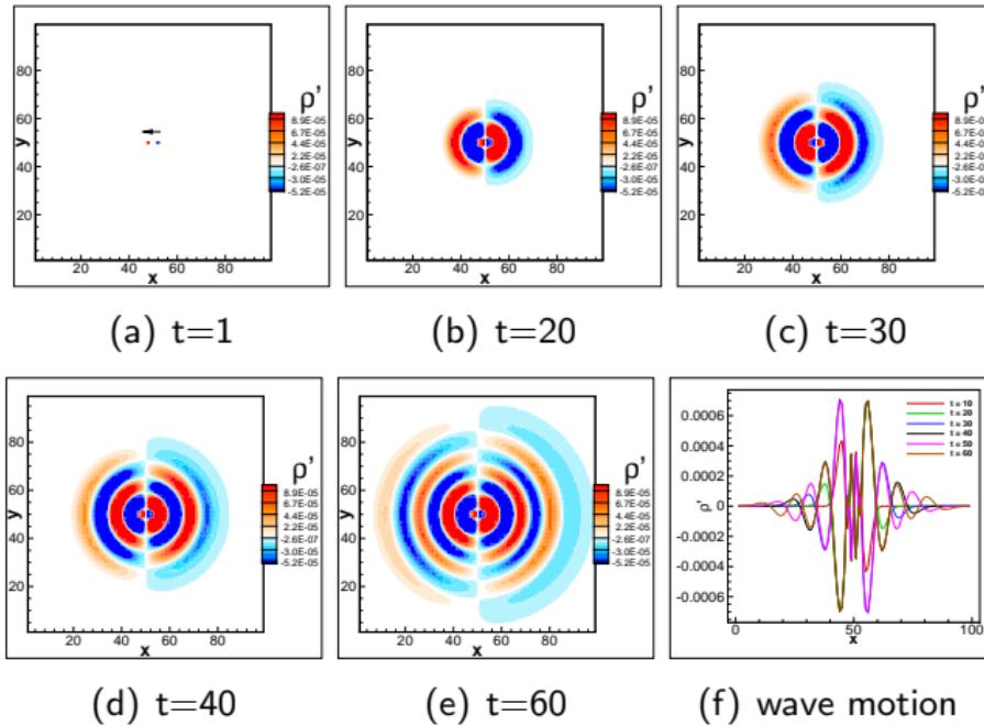
Figure: Propagation of density perturbation waves for the case of a dipole
