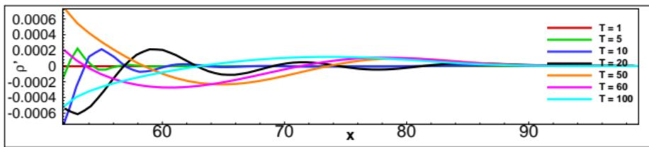
Figure: Propagation of density perturbations for different time periods of excitation
