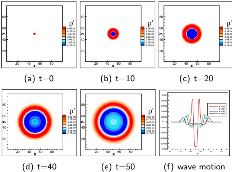
Figure: Propagation of density perturbation waves for the case of pulse
