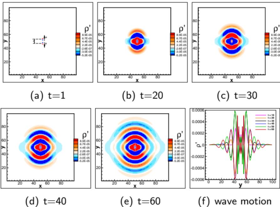
Figure: Density perturbation waves for the case of a longitudinal quadrupole
