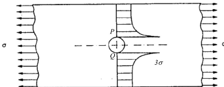
Fig.5. Radial distribution of hoop stress components  $\sigma_{\theta\theta}$  along the ligament where  $\theta = \pi/2$
