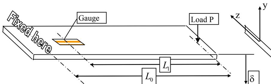
Fig. 2 Important dimensions and Co-ordinate system axes
