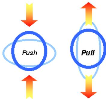
Fig. 2 Schematic diagram of the changes in the ring diameter as compression (push) and tension (pull) forces are applied.
