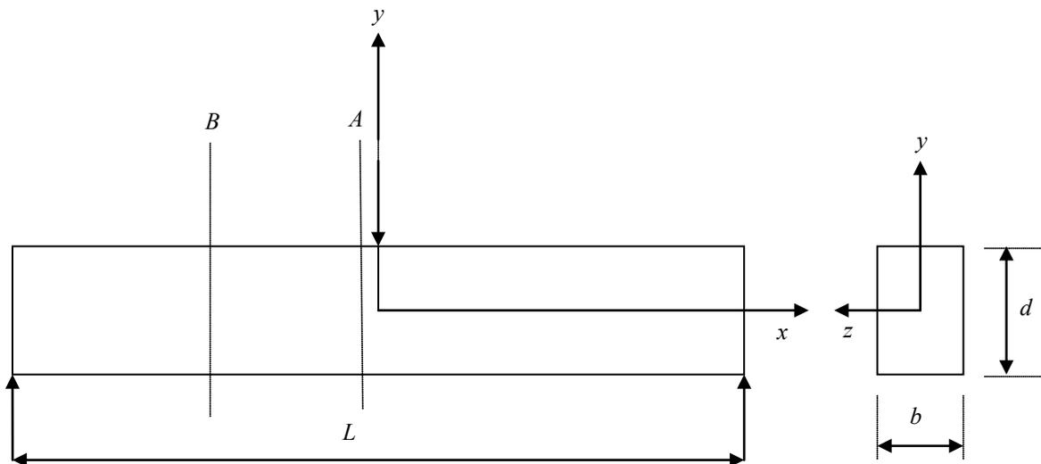
Fig. 1. Beam under three point bending
