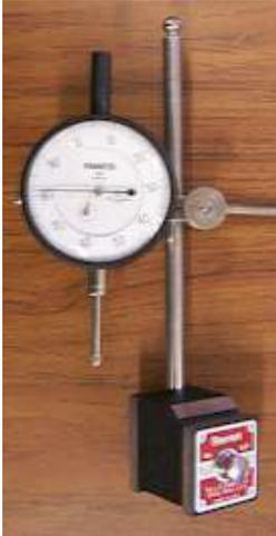
The gage shown in the figure has a smallest increment of one thousandth of an inch (0.001), and can move 1 inch. Precision is listed as  $\pm 0.0005$  inches.
