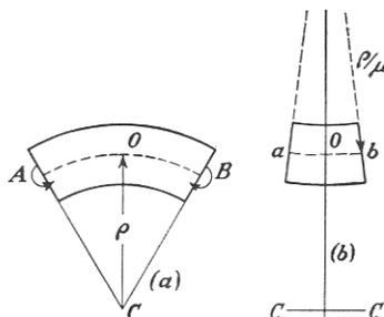
He demonstrates that these two assumptions are rigorously fulfilled only in four-point bending. He also shows that the initially rectangular cross section changes its shape as shown in the figure having anticlastic curvatures due to lateral contraction of the fibres on the convex side and expansion on the concave side.
