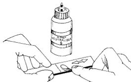
Fig. 4 Scrubbing the surface with cotton tipped applicator
