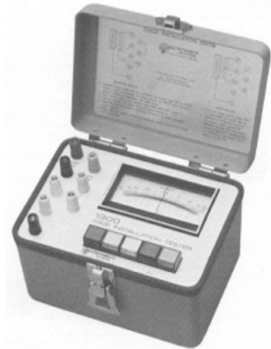
Fig. 17 Model 1300 strain gage installation tester
