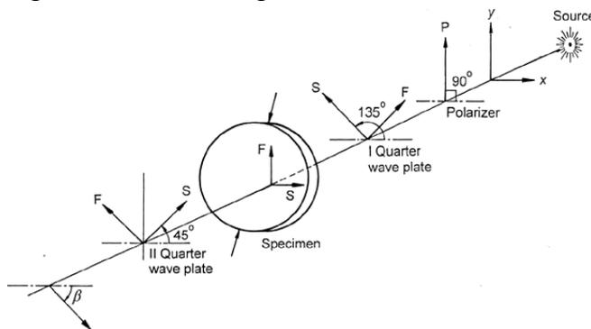
Fig. 1. Arrangement for Tardy's method of compensation
