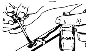
Fig. 15 Application of protective coating
