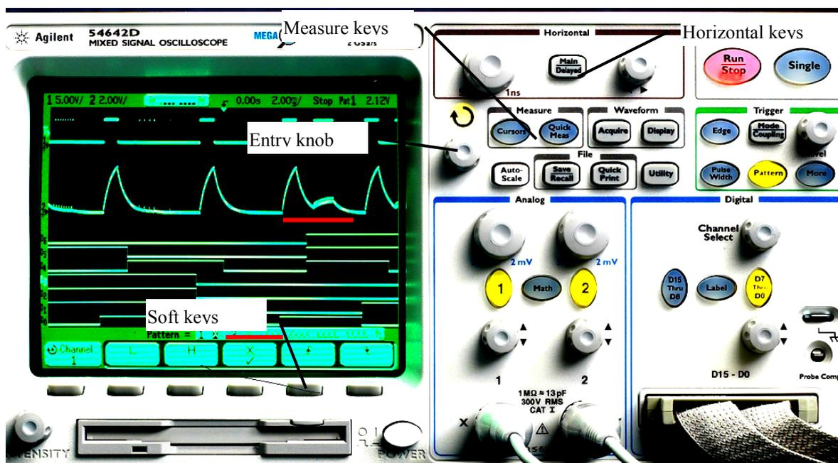
Values like frequency, period, voltage levels of waveforms ( $\Delta x$ ,  $\Delta y$  etc) can be easily measured using cursors. Cursors are horizontal and vertical markers/gridlines that indicate X-axis values (usually time) and Y axis values (usually voltage) on a selected waveform.
