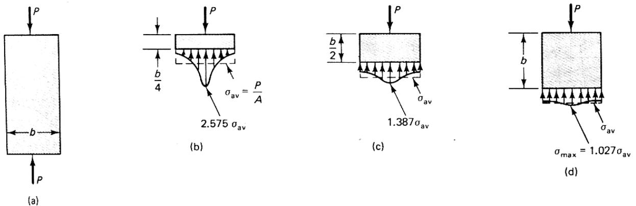
Consider that a uniformly distributed load needs to be applied to a bar as shown. Instead a concentrated load which is statically equivalent is applied at the end. The rigorous solution to this problem by theory of elasticity reveals that the loading becomes uniform at a distance  $b$ , which is the thickness of the specimen. Closer to the loading one cannot estimate the stress by invoking  $P/A$ . This can be done only beyond  $b$ .
