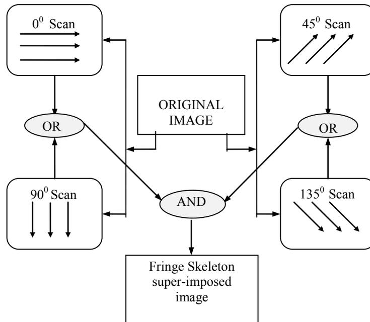
Fig. 1. The scheme of logical operators to obtain continuous fringe-skeleton
