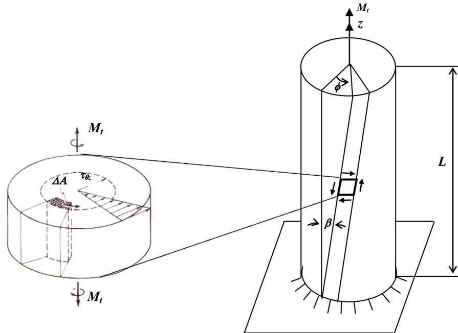
Fig. 3 Figure showing the definition of angle of twist
