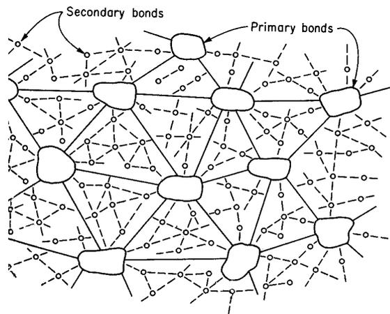
Fig. 1. Primary and Secondary molecular chains in Diphasic Polymer
