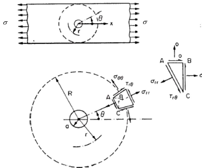
Fig.3 Stress distribution around a circular hole
