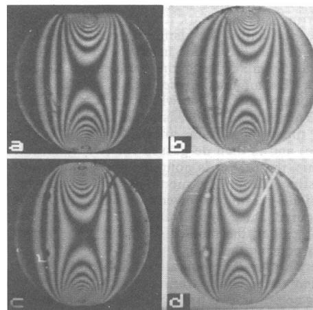
Fig. 2. Isochromatic observed for a stress-frozen disc, the fringes are not distorted after introducing two holes and slot
