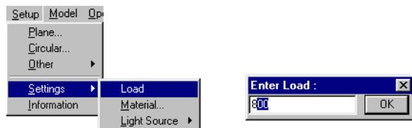
Fig. 3. Procedure for changing the load applied
