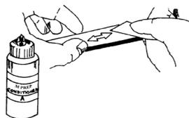
Fig. 2 Surface Abrading
