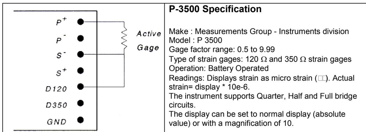
Fig. 5 Strain Measuring Bridge (instrument) Front panel, Quarter-bridge circuit connection details and P-3500 specifications.
