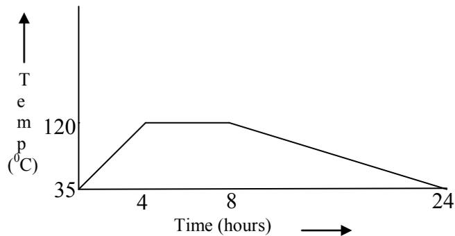
Fig. 3. Temperature Cycle for *stress freezing*
