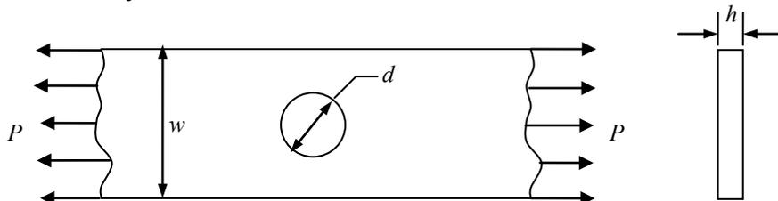
Fig. 2. Plate with a discontinuity (hole)
