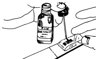
Fig. 7 Catalyst application (Step 1)
