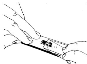
Fig. 11 Removal of cello tape (Step 5)
