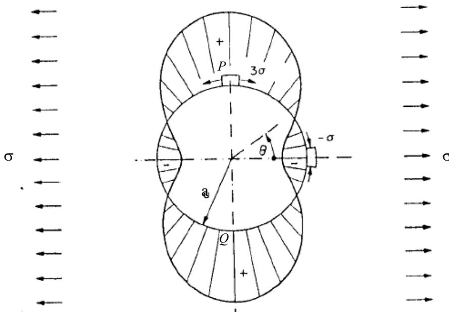
Fig. 4. Distribution of hoop stress  $\sigma_{\theta\theta}$  around the circumference of circular hole in a large body
