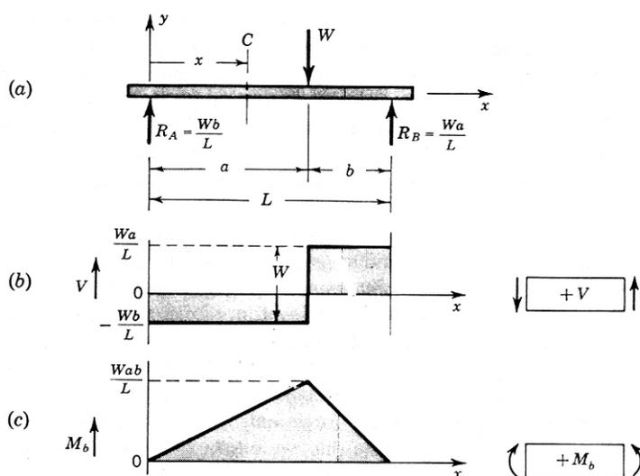
Force or moment in the positive direction on the positive face is positive and on the negative face the negative direction of these is considered positive. This sign convention is in tune with the general sign convention mentioned previously.
