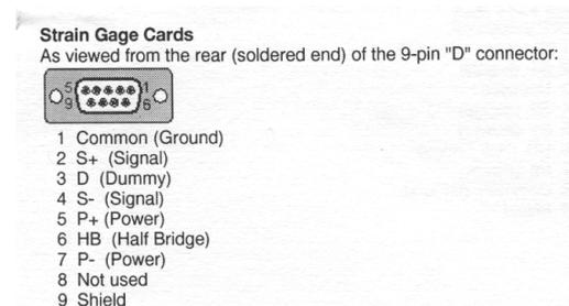
Scanner card is pulled out and the dummy resistor jumper is moved to the corresponding place according to the resistance of the strain gage (120/350/1000 ohms) used. This is useful in shunt calibration
