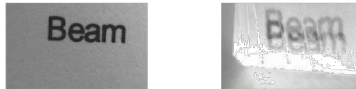
Fig.1 Double Refraction in a Calcite crystal
