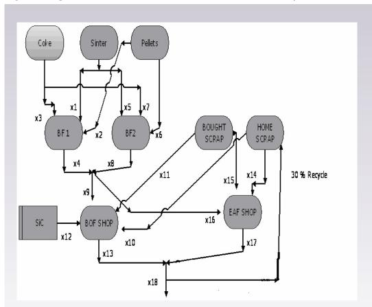
Fig. 2: Schematic layout and material flow in the primary end of an integrated steel plant
