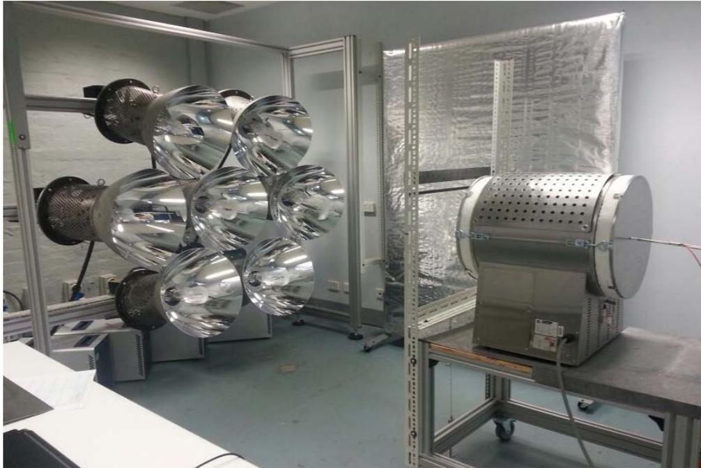
42 kW Solar simulator and reactor at Swinburne
