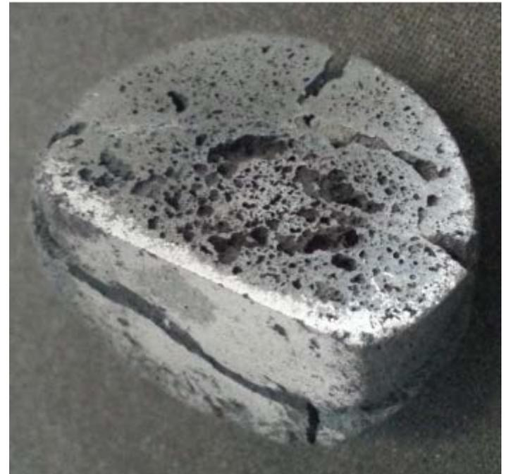
Partially reduced iron ore composite pellet
