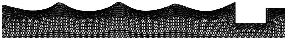
**Fig. 5.22 Typical Mesh Configuration in the Presence of a Rectangular Object**
